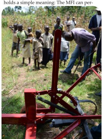
form a variety of functions like ripping, chiseling, and weeding all at once. The tool is animal-drawn, and the farmer using it can switch applications quickly and safely.
