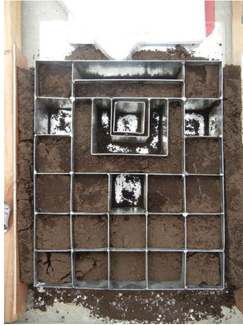
Cookie-cutter device made by R. Parra used for sampling greenhouse experiment.
