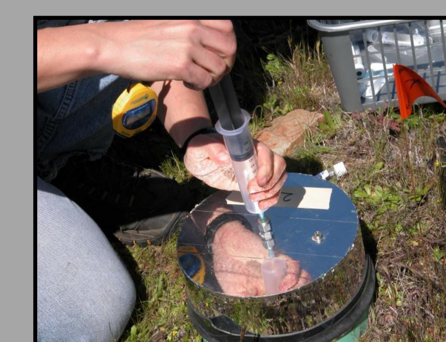
Sampling soil gases for carbon dioxide, nitrous oxide, and methane quantification.
