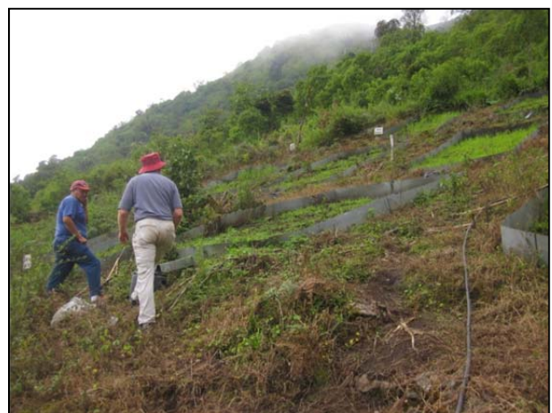
Figure 2. Runoff plots at the Rio Alumbre site.
