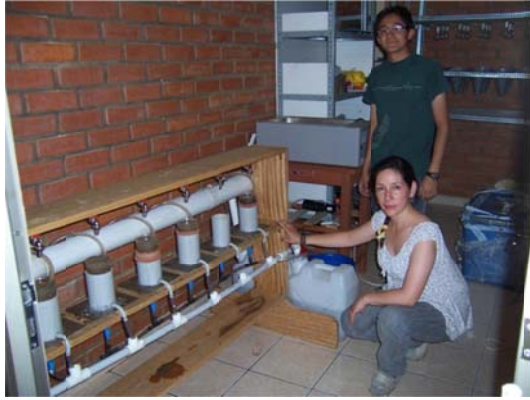
View of completed K_{sat} device on left and completed soil moisture tension table on right. Tension table is shown with a single soil core. It can accommodate at least six cores.
