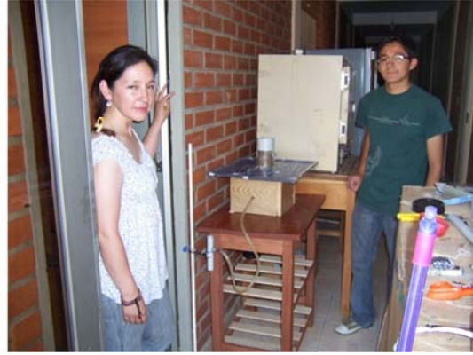
View of completed K_{sat} device on left and completed soil moisture tension table on right. Tension table is shown with a single soil core. It can accommodate at least six cores.
