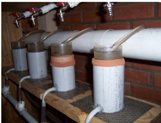
Detail of K_{sat} device showing maintenance of constant water head on intact soil cores via siphon tubes from constant water level trough.
