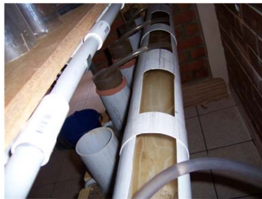
Detail of K_{sat} device showing maintenance of constant water head on intact soil cores via siphon tubes from constant water level trough.
